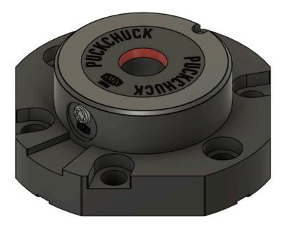
begin spinning the rotary table and tapping the receiver with a mallet to align the center of this bushing with the centerline of your rotary. Gradually tighten the mounting bolts as you go until they are fully tightened (as high as 60 ft-lbs for ½-13 or M12 t-nut threads). *Neither the outside diameter of the puck nor the receiver base are precision surfaces, it is recommended to only use the center tapered bore for centering the receiver.*
