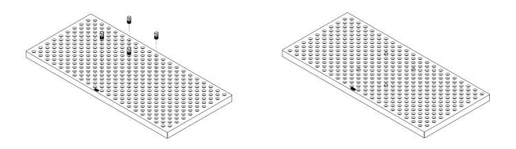
Place the 'locating' receiver onto its pin. Ensure the pneumatic fitting (Automatic PuckChuck) or clamping screw (Mechanical PuckChuck) is facing in the desired orientation. Install but **do not fully tighten** the four mounting screws.
