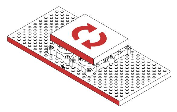
If the pallet extends past the receiver Puck diameter, this will require either clearance features through the pallet or low profile (a.k.a. 'Short-arm' or stubby) hex wrenches to access the mounting bolts. If the desired tram is not reached the fixturing pin below the 'diamond' receiver may need to be removed before tramming.
