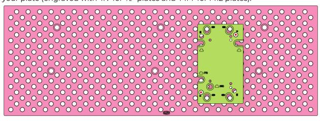
3. Install **locating pins** in the two locations noted in the last step. We recommend SMW fixturing pins but off-the-shelf dowel pins are acceptable.
