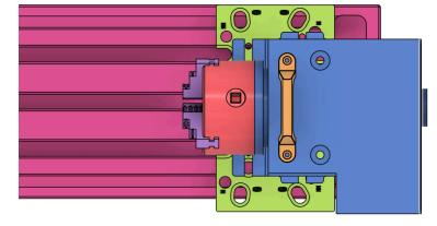
5. Install the **four 5/16-18 x 1**<sup>3</sup>/<sub>8</sub>" **socket head cap screws** and washers into the threaded holes in the above step. Before tightening ensure the rotary is positioned as desired.
