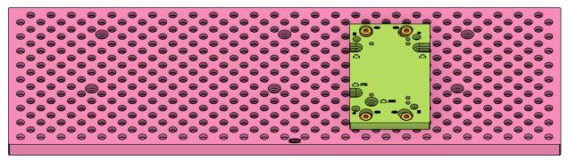
6. Place the **microARC** on top of the **subplate**, aligning the mounting slots with the 5/16-18 threaded holes on the subplate. For this mounting case you will be using the **four holes highlighted below**. Note: we recommend a light coat of dielectric grease or corrosion inhibitor between the rotary and subplate.
