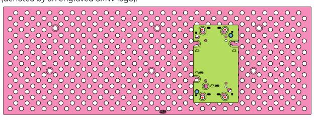
5. Install the **four low-profile socket head screws** (½-13 x 1.0" or M12 x 25mm) into the four holes noted in the previous step. See **this page** for torque specifications for your specific **fixture plate**.
