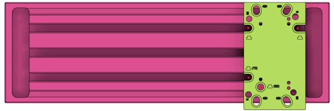
Install the three t-nuts and secure the subplate with the ½-13 x 1" low profile screws. Tighten the bolts to 60 ft-lbs [81 N-m]. Note: to allow for adequate alignment of the microARC, this should be trammed to your machine axis within approximately 0.01" [0.25mm].
