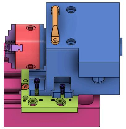
Once in place, lightly snug these screws. Do not fully tighten.
