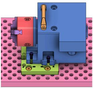
Once in place, lightly snug these screws. Do not fully tighten.
