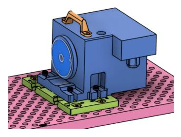
Installation is complete. When ready to remove the rotary, leave the 5/16 screws in place, loosen the ½-13 or M12 screws, and remove the rotary + subplate as a unit. Re-installation is as simple as installing the subplate back over the locating pins and tightening the mounting bolts.
